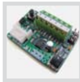
P111408 - SCS WIE Circuit board for direct connection of wiegand accessories (such as SELETTO, COMPAS SLIM, etc) to the control units QSC D MA, LIBRA C MA, LIBRA C MV, LIBRA C LX, VENERE D, LEO D MA, LEO MV, RIGEL 5 and ALTAIR P.
