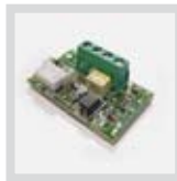
P111376 - SCS 1 Serial connection board for QSC D MA, LIBRA C MA, LIBRA C MV, LIBRA C LX, VENERE D, LEO D MA, LEO MV, RIGEL 5 and ALTAIR P.
